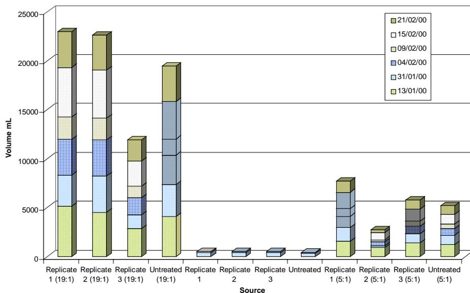
Figure 17 Leachate volumes measured from lysimeters with (a) a 19:1 loading, (b) no loading and (c) a 5:1 loading
