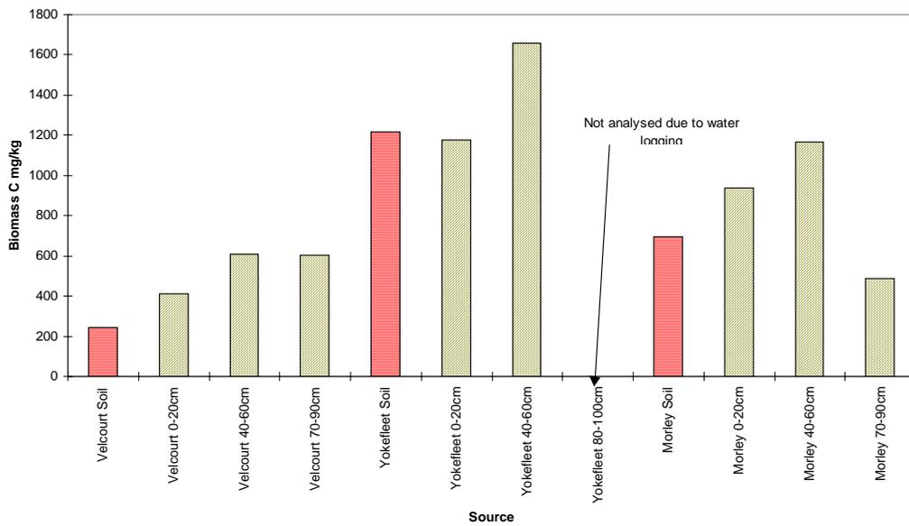
Figure 4 Total biomass measured in samples taken from the three biobeds as well as the soil component of the biomix, 16 - 45 days after construction
