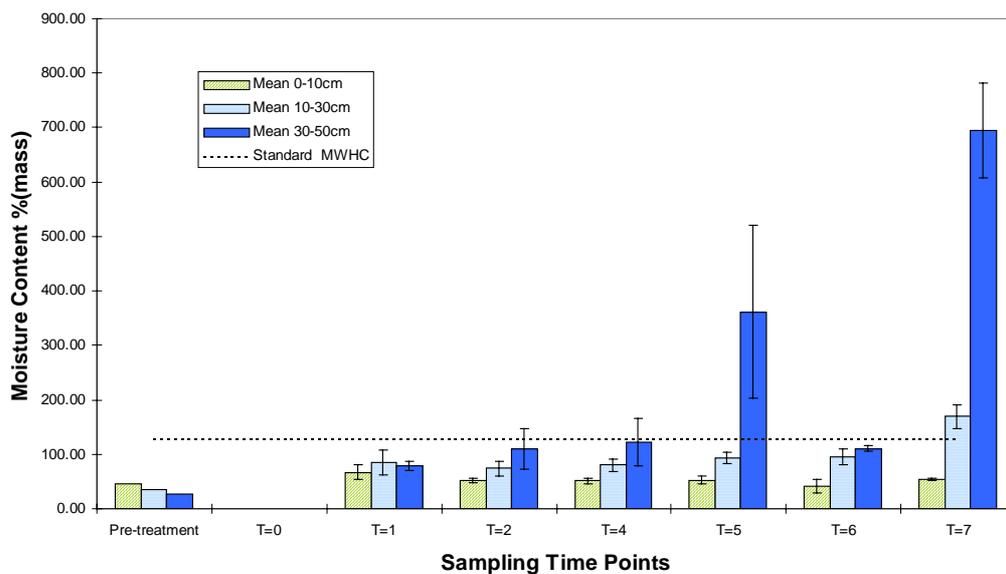
Figure 5 Measured water content within the biobed cores
