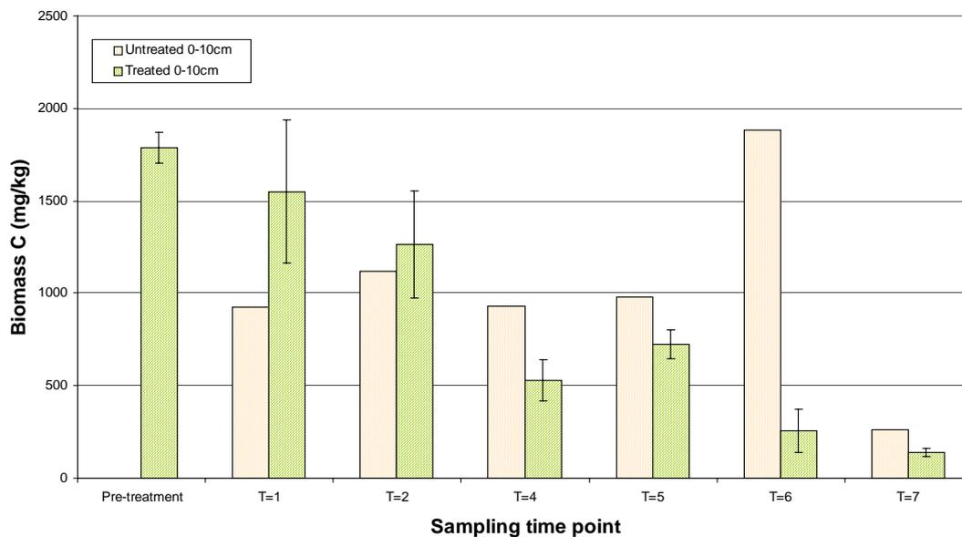
**Figure 6 Mean biomass in the 0-10 cm layer of the closed biobed columns**
