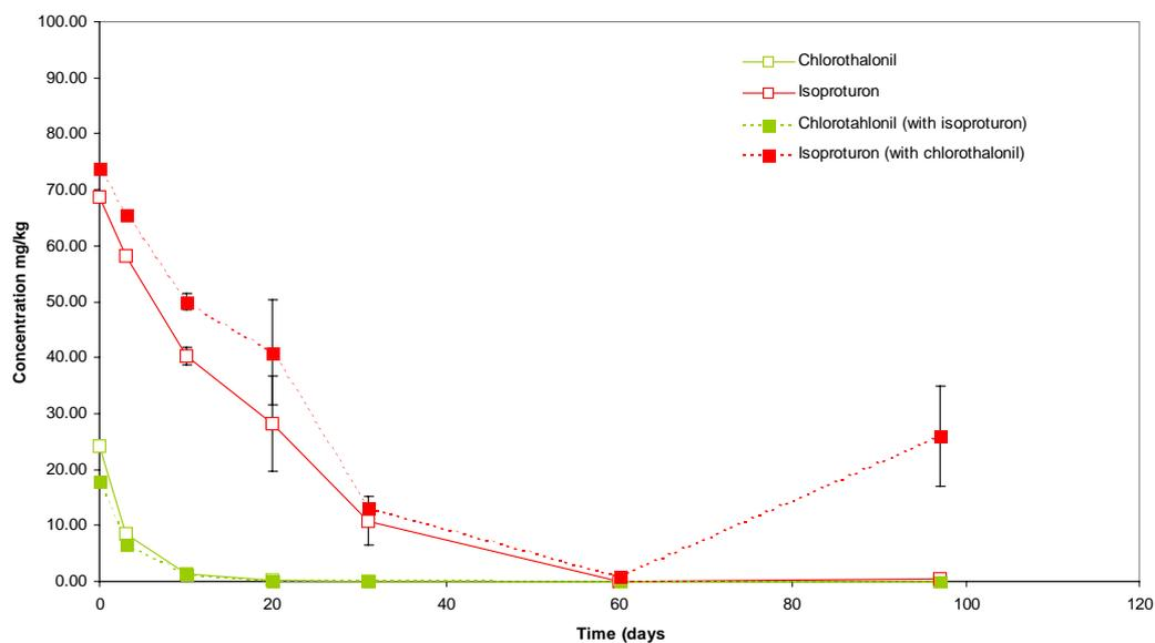
**Figure 24 Isoproturon and chlorothalonil degradation individually and in combination in biomix**
