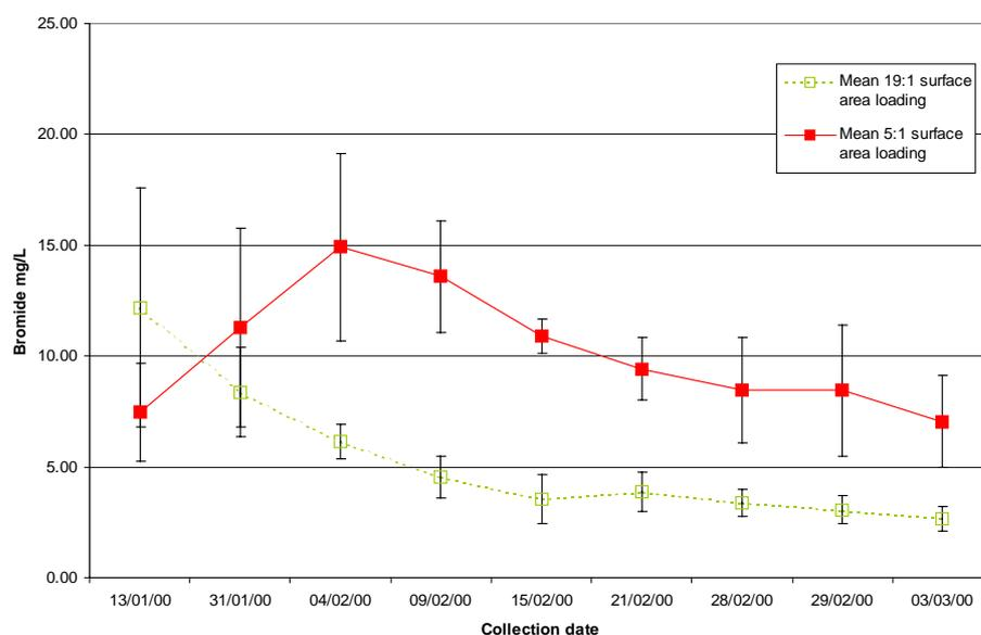
**Figure 18 Bromide breakthrough in lysimeters with a 19:1 and 5:1 surface area loading**
