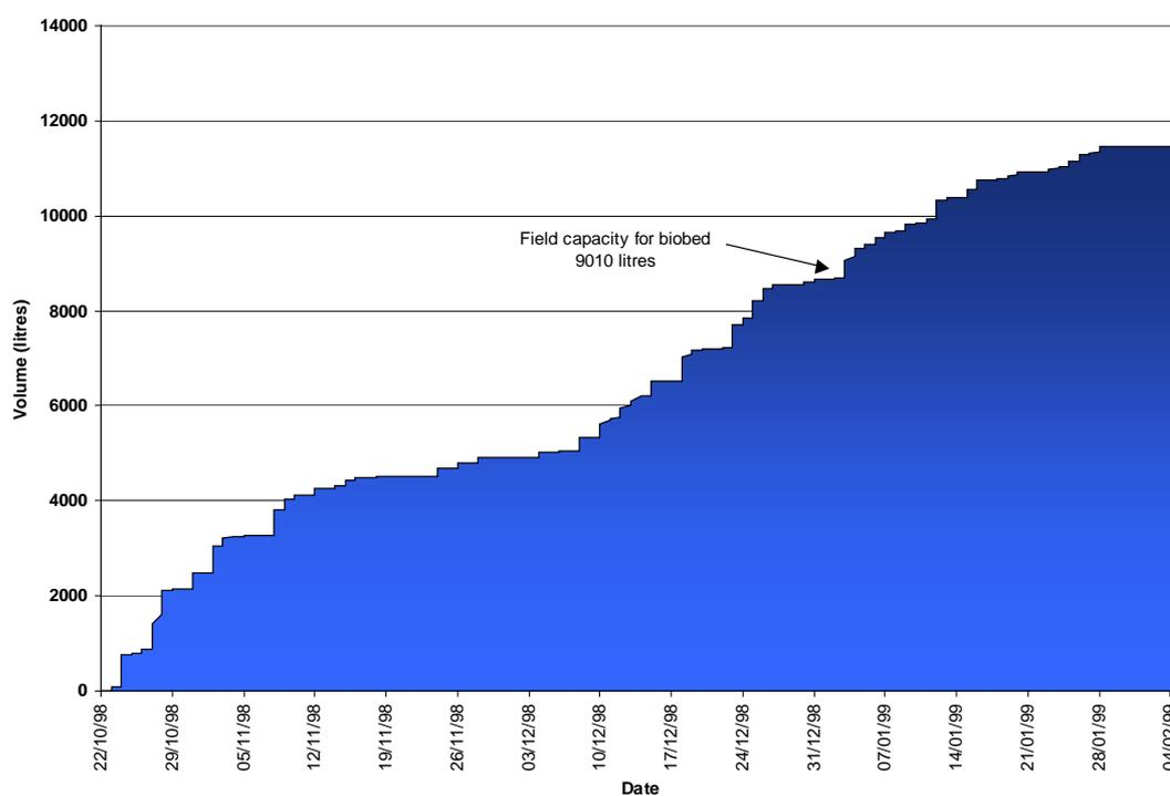
**Figure 2 Volume of water intercepted by the Morley biobed prior to being covered**
