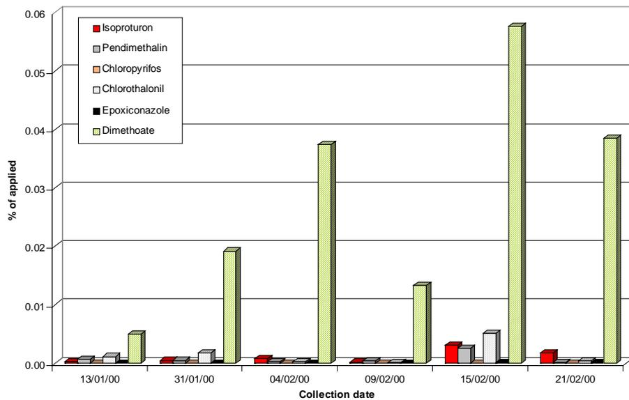
Figure 22 Pesticide residues in leachate (as a % of the applied) from lysimeters with a 5:1 loading
