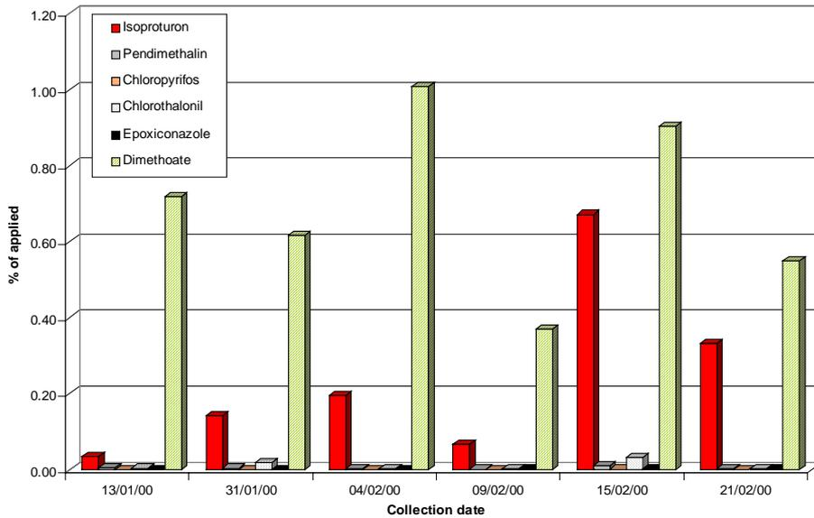
Figure 21 Pesticide residues in leachate (as a % of the applied) from lysimeters with a 19:1 loading
