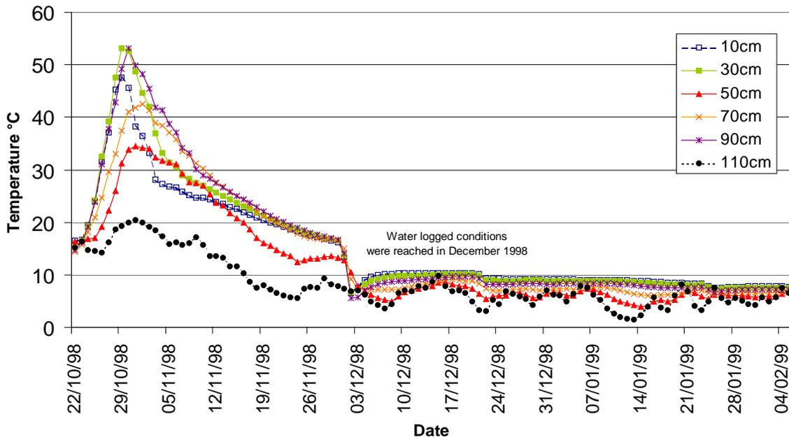
Figure 3 Average temperatures recorded at different depths in the biobeds situated at Morley
