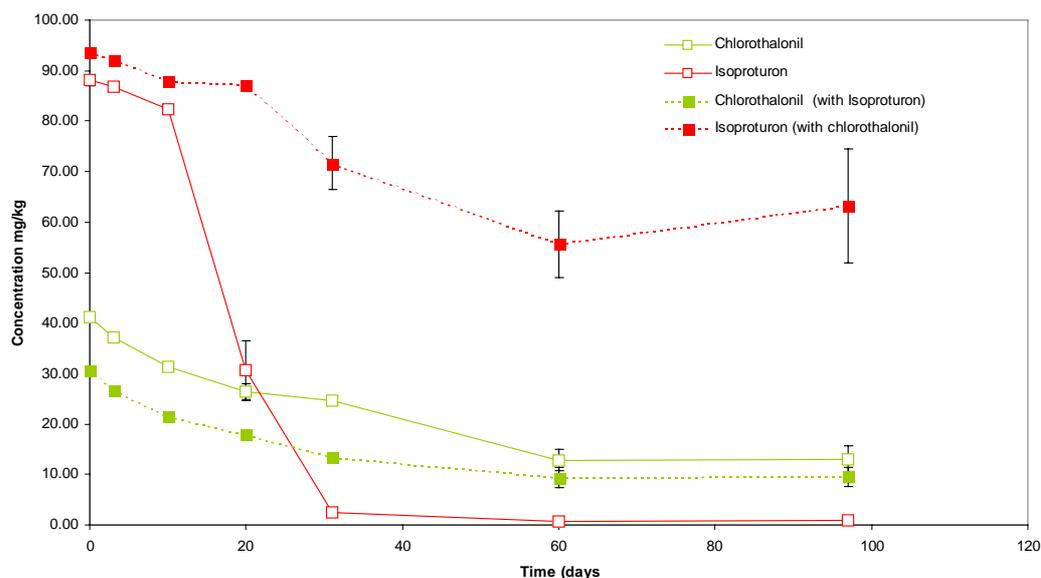
**Figure 25 Isoproturon and chlorothalonil degradation individually and in combination in topsoil**
