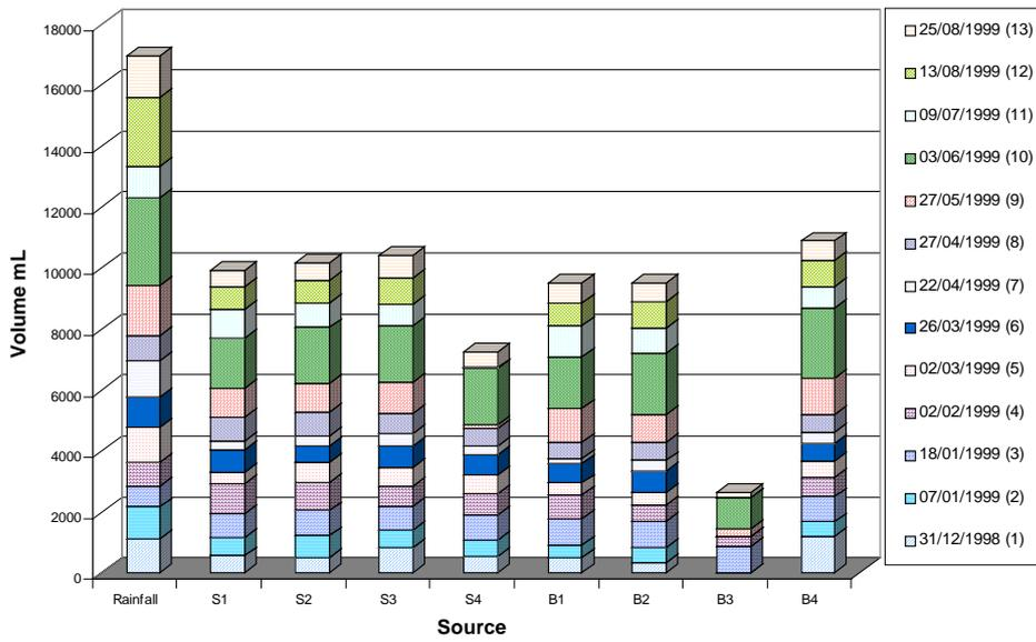
Figure 10 Leachate volumes measured in soil cores (S1 - S4) and biobed cores (B1 - B4)
