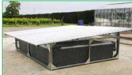
'Treatment' of spray washings is offered by one system which relies totally on evaporation to reduce the collected liquid to a residue held within a plastic liner. Thus no discharge is made from the system.
