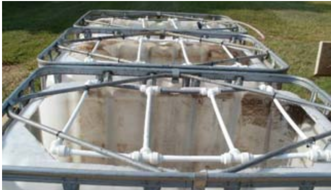
Three IBC's complete with drilled and secured spray bars
