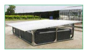
'Treatment' of spray washings is offered by one system which relies totally on evaporation to reduce the collected liquid to a residue held within a plastic liner. Thus no discharge is made from the system.
