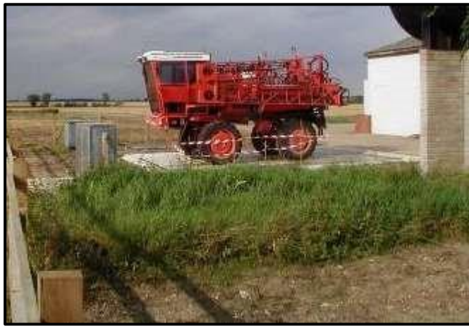
Indirect biobed. Sprayer is parked on impermeable handling area with runoff diverted onto an adjacent biobed
