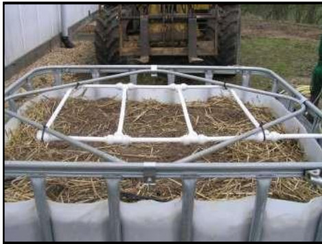
DIY Biofilter pipework
