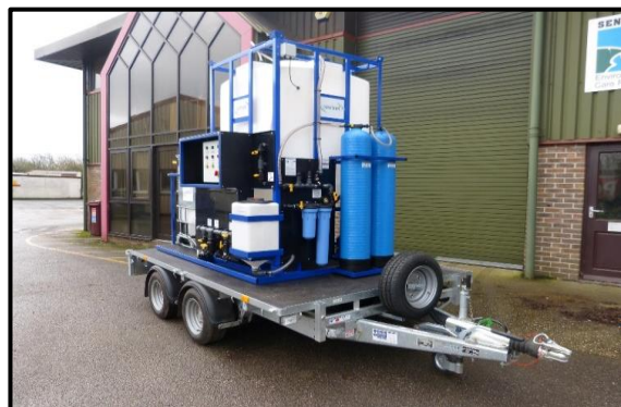
A mobile treatment unit
