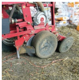
Fill drills in areas where spills can be cleared up
